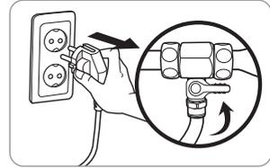
2. Please empty the water tank completely using the draining hose after pressing and letting down the front draining door.
