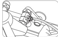
5. Open the feed valve to supply water to the filtration system.
