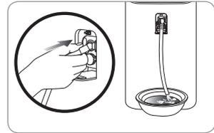
3. Please remove the top cover, and then un-hook the fixed clip holding the top cover of the water tank. Now remove hose and open the tank cover.
