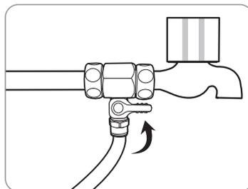
2. After separating the fitting connected to the filter to replace, please replace the filter. (Separate the fitting using the proper tool.)
