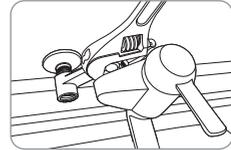
2. Apply the teflon tape on the adaptor and fit it to the pipe.
