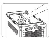
6. Rinse the interior water storage tank clean with water taken in advance from the machine, and then use the outlet tubing to completely drain. Run purified water through the product once and empty, and then use.
